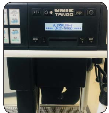
Restart the machine and verify operation by making a few drinks
