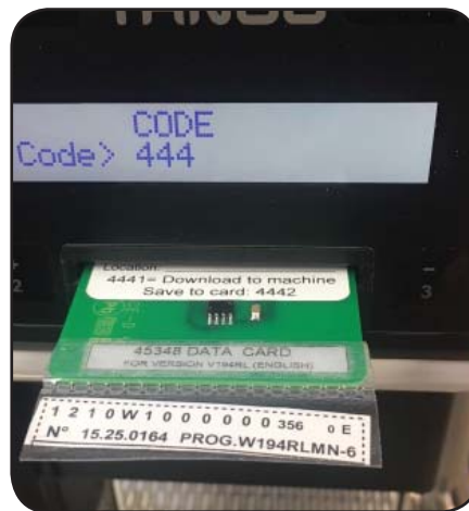
Re-insert Memory Cards and enter 4441 to down- load drinks into machine
