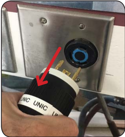
Unplug machine and wait 1-2 minutes
