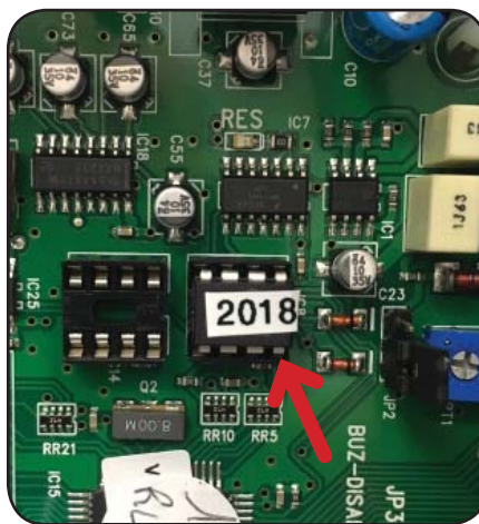
Gently press the new chip in-place
